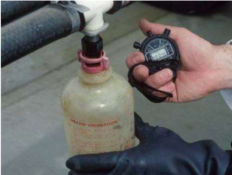
A stopwatch used to calibrate a sprayer prior to an application of herbicide (NRCS Photo Gallery NRCSMD91001)
