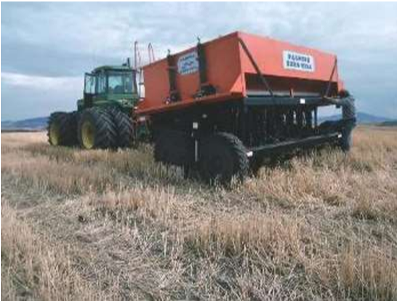
Large no-till planters used in Washington's Palouse region (NRCS Photo Gallery NRCSWA84002)
